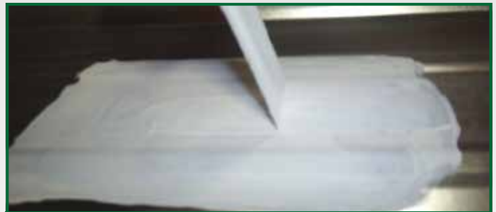
Step 6: Pull polyester fabric at a 90° angle to verify cohesive (pass) or adhesive (potential fail). Picture shows cohesive failure.
